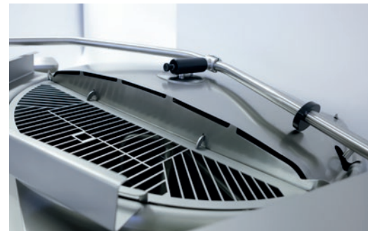
Safety grid lid for safe operation.
